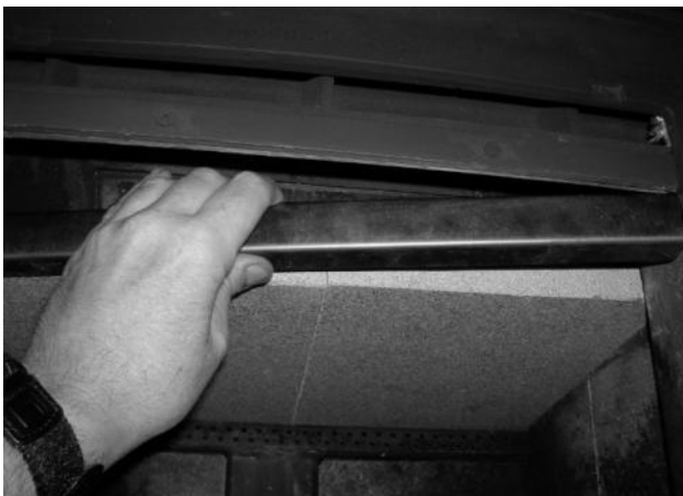
Figure 16 - Removing/Replacing the Baffle for Inspection
